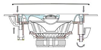
6) After the screws are tightened and the speaker is level with the ceiling, the front grill can be assembled to the loudspeaker.
